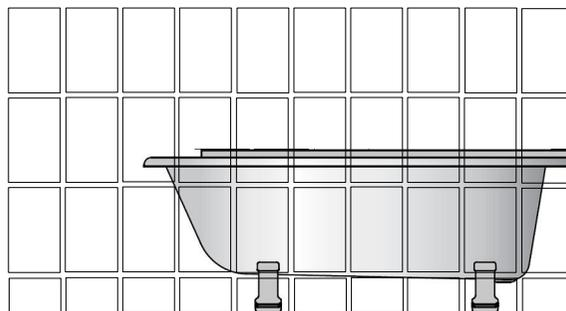
Tiles are cut to provide slot for bath to fit into. The cut in the last tile will need to be shaped to accept the corner detail of the bath rim.
